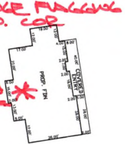
PROP. FOUNDATION DETAIL SCALE: 1"=4'-0"
